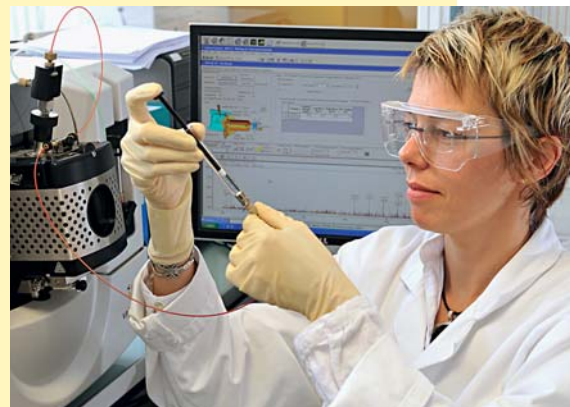
Estelle Gueneau, Annemasse Analytical Laboratory Manager, injects a material sample into the GC/MS gas chromatograph.
