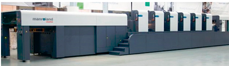
The new Man Roland B1 707 LTTLV Evolution at Pyroll Takon Kotelotehdas Oy in Tampere (with 7 color units & 2 lacquer units, supplemented with UV).
