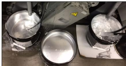
*SICURA FLEX LED SILVER on left & competitive silver on right extended 40% to resist foaming. Photo taken 1 hour after running.*
