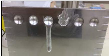
*Same product on a flow meter to illustrate SICURA FLEX LED 877 SILVER's ability to maintain flow during a run.*
