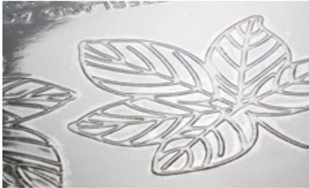
The varnish has an approximate relief height of 250 µm. It dries excellently, remains flexible and shows no yellowing.
