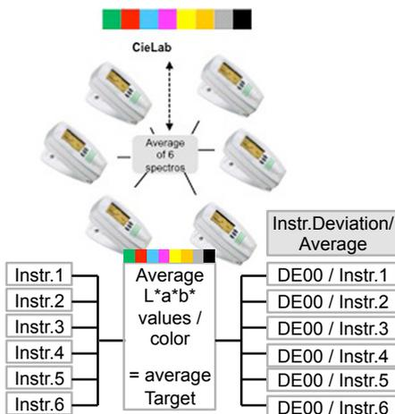
The global average deviation is consistent with the manufacturer's specifications. Usual tolerances applied for color matching (DE00 ≤ 1) are 5 times wider than average inter-instrument deviations. This guarantees a good level of security.
