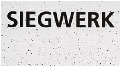
Left: white with pinholes, right: optimised white without pinholes
